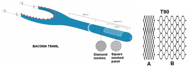
Figure F.4.4.1. Idealized picture of the Bacoma trawl and T90 Codend. (Modified from Swedish Board of Fisheries website: <a href="http://www.fiskeriverket.se/laboratorier/havsfiske/publikationer.htm">http://www.fiskeriverket.se/laboratorier/havsfiske/publikationer.htm</a>)
